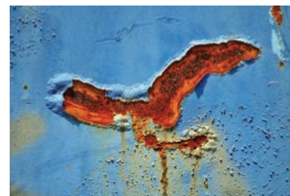
▲ A scratch in paint often allows the underlying iron to rust.
