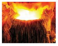
▲ Blast Furnace Molten pig iron reacts with a "blast" of oxygen gas that converts carbon and sulfur impurities into  $CO_2$  and  $SO_2$  gases.
