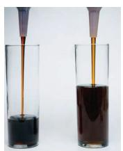
▲ Viscosity The motor oil on the left is more viscous and flows more slowly than the motor oil on the right.
