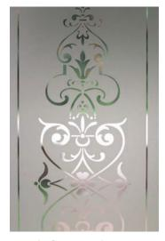
▲ Hydrofluoric Acid, HF Although aqueous HF is a weak acid, it attacks glass. This design was created by coating glass with wax and then removing wax from the pattern areas. The glass was dipped into hydrofluoric acid, which etched the design.
