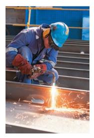
▲ Oxyacetylene Welding The reaction of oxygen and acetylene gases releases enough heat to melt iron.
